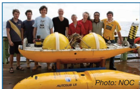
Autosub Long Range, after its successful trials. Top panel removed, to show the two main pressure spheres (forward – battery, aft – control system, ADCP). Members of the onboard engineering team: Alex Phillips, Maaten Furlong, Miles Pebody, Steve McPhail, Peter Stevenson, James Perrett, Mario Brito and Leo Steenson.
