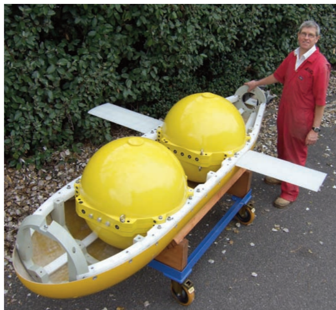
Peter Stevenson, the AUV team chief mechanical engineer, with the Autosub Long Range AUV. The top half panel has been removed, revealing the two spherical pressure housings which hold the control electronics and batteries. The wings allow the AUV to cope with buoyancy changes as it dives to depths of up to 6000m. Photo: Steve McPhail, NOC
