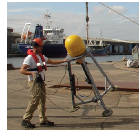
Steve Mack with a MYRTLEX capsule in a test frame during trials at Vittoria Dock, Birkenhead.
