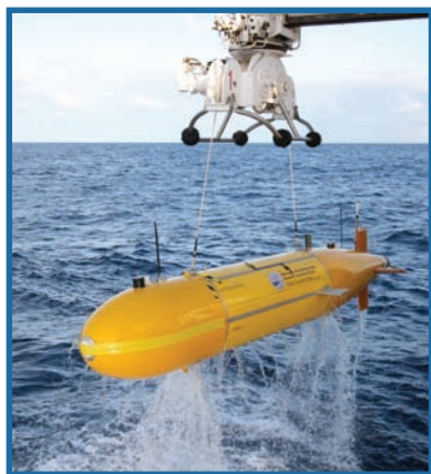
Autosub6000 lifted into its recovery cradle following its first deep mission. (Image by Maaten Furlong)
